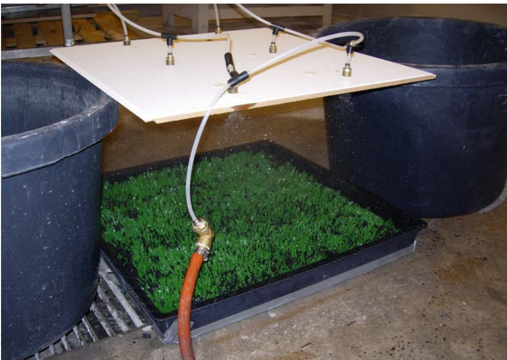
Figure 3.1 Arrangement for spraying the test specimen with water
